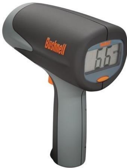
Figure (4): Instrument used to measure vehicle speed at work zone
