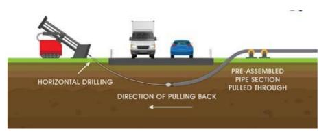
Figure 4: Horizontal Directional Drilling [10]
