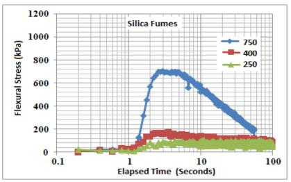
Figure 3. Variation of flexural strength under various microstrain levels of silica fumes treated mixture
