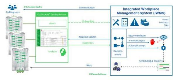
Diagram 2: IWMS Smart Buildings data flow diagram
