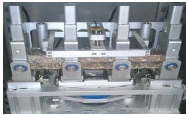
Figure 1. Four points flexural bending test setup.
