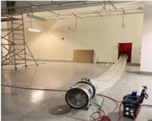
Fig 5. Pressurizing exterior wall
