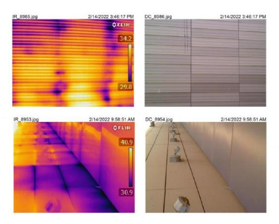
Fig 2. Thermal scan of Building Envelope
