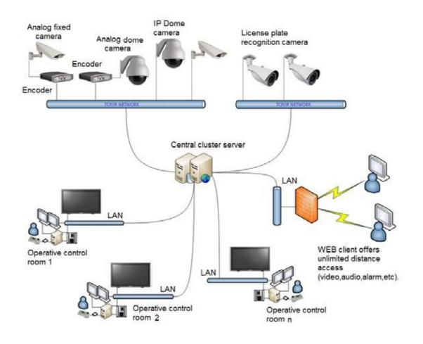
Figure 2: Closed-circuit television (CCTV) Surveillance Systems for Building
