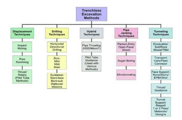
**Figure 3: Trenchless Construction and Excavation Methods**
