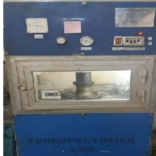
Figure 3. Repeated compressive stress test
