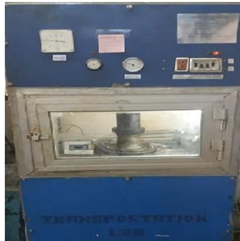
Figure 3. Repeated compressive stress test
