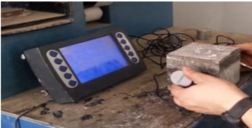
Figure 4. Ultrasonic wave test process
