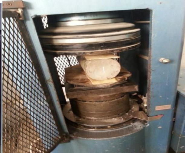
Figure 7. Indirect Tensile strength test
