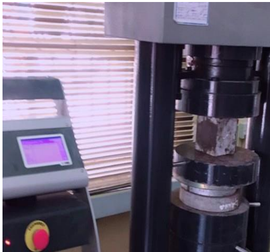
Figure 6. Compressive strength test
