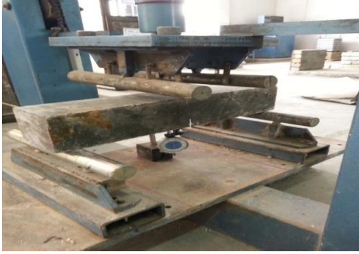
Figure 9. Flexural strength test
