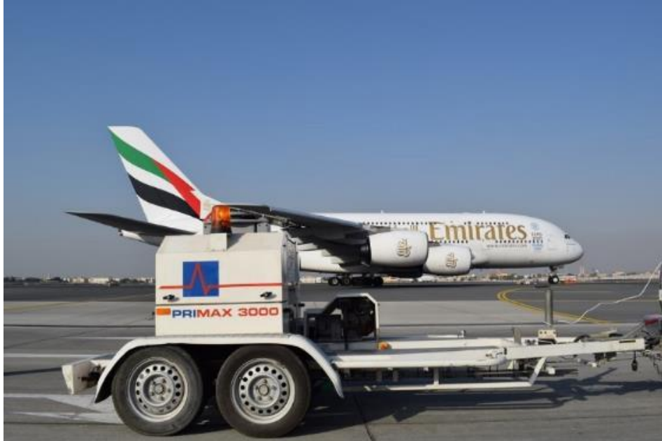
Photo 1: Used SH-FWD in pavement structural evaluation.
