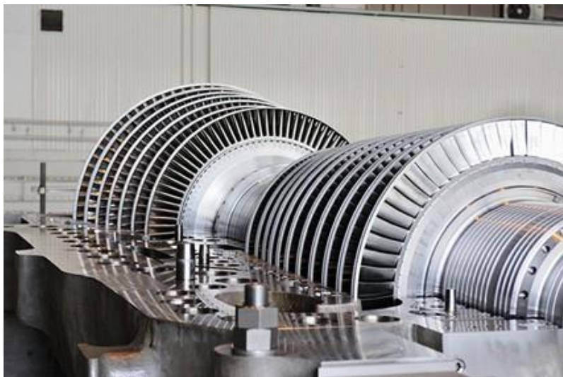
Figure 1 472-megawatt steam turbine generator (photo credit: businesswire.com)
