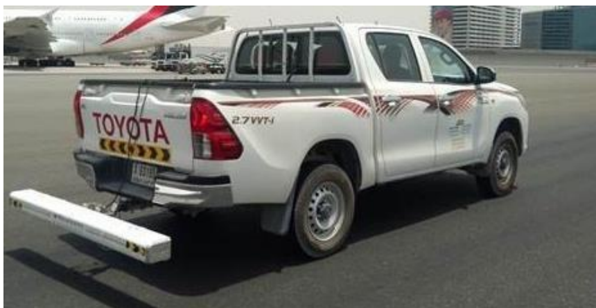
Photo 2: Used Laser Profiler in pavement roughness evaluation.
