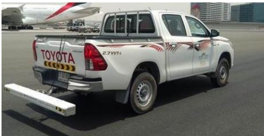
Photo 2: Used Laser Profiler in pavement roughness evaluation.
