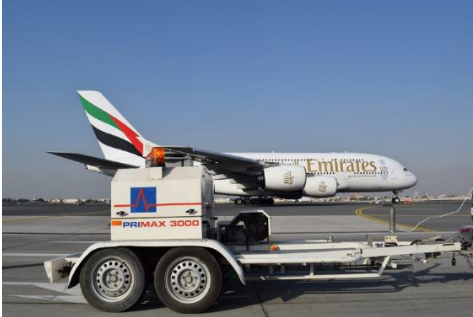
Photo 1: Used SH-FWD in pavement structural evaluation.
