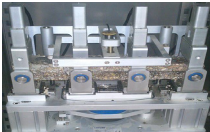
Figure 1. Four points flexural bending test setup.
