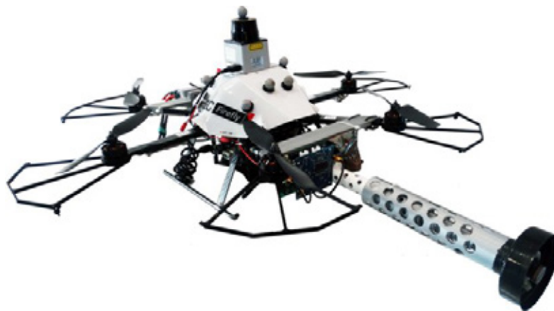
Fig. 5 Example of a Drone (UAV) equipped with an NDT system [16]
