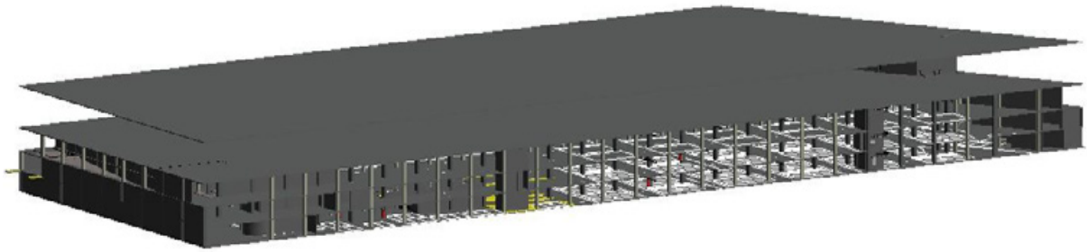
Figure 3: BIM final model of the car park of commercial building for Maintenance and FM purpose
