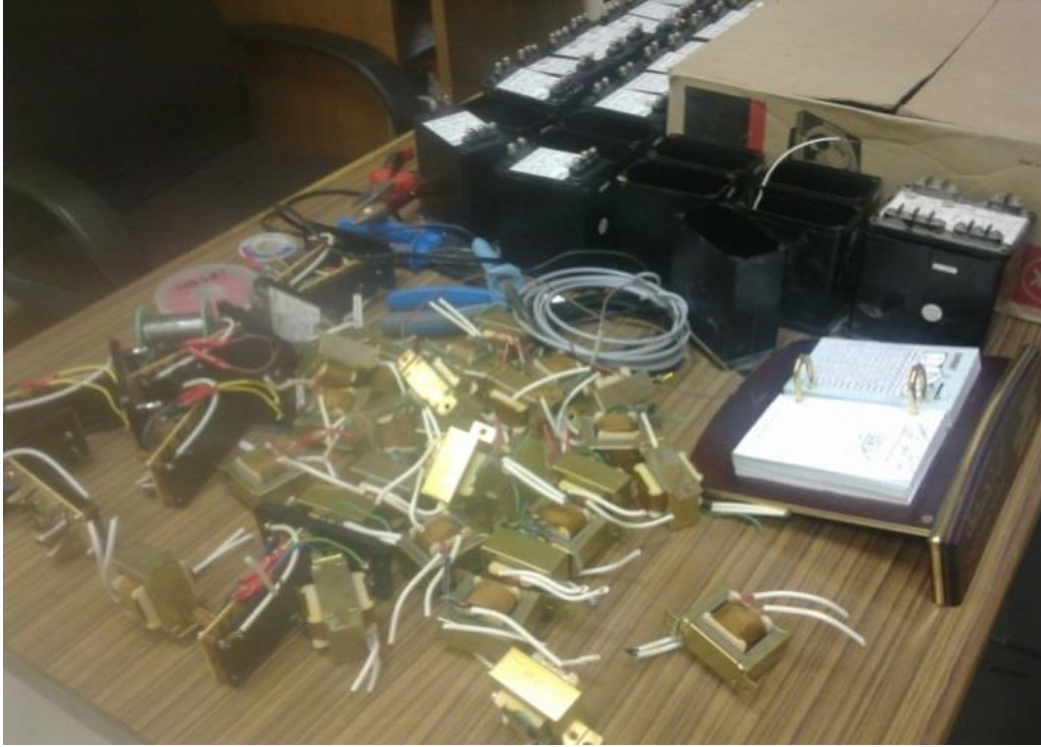
Figure .7: Old & released transducers being modified for DC system voltage monitoring
