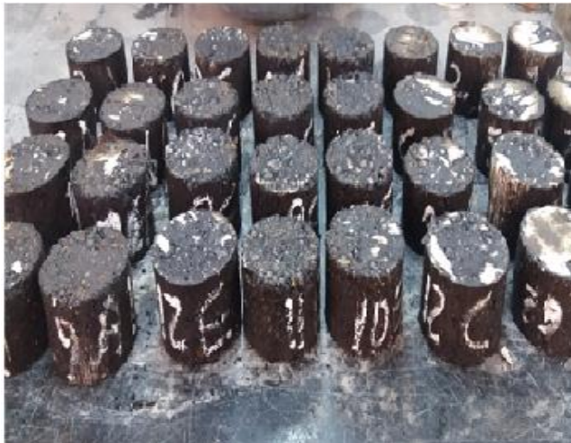
Figure 2. Part of recycled asphalt concrete specimens
