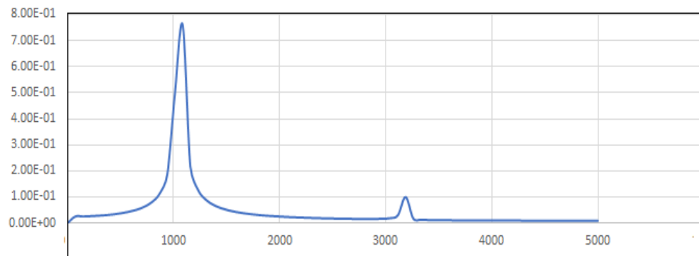
Figure 11. Vibration Response of Pump Casing
