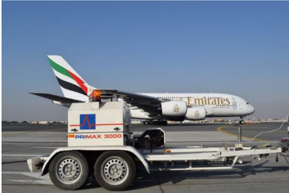
Photo 1: Used SH-FWD in pavement structural evaluation.
