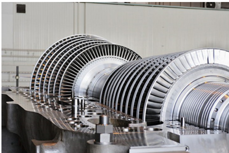
Figure 1 472-megawatt steam turbine generator (photo credit: businesswire.com)
