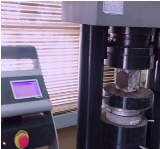
Figure 6. Compressive strength test
