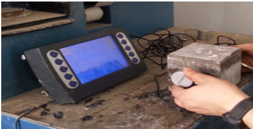
Figure 4. Ultrasonic wave test process
