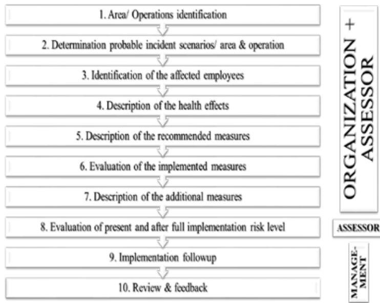
Figure 1: The improved 10-step Risk Assessment Study approach that must be used for industrial and other high-risk operations
